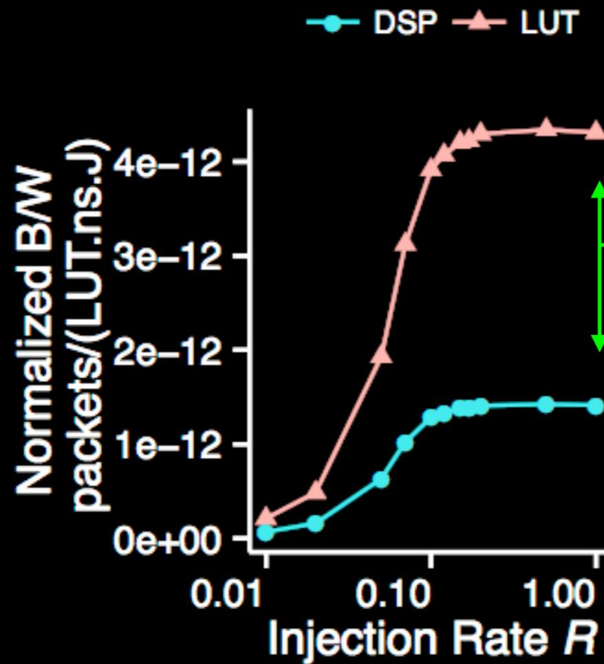
*DSP48s less-efficient than LUT-based Hoplite!*
